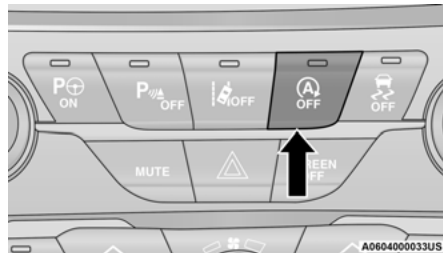
Stop/Start OFF Switch
