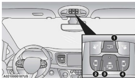
Overhead Console Power Switches
