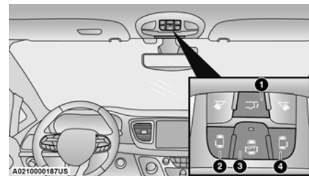
Overhead Console Power Switches
