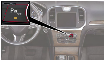
Parksense Switch Location
