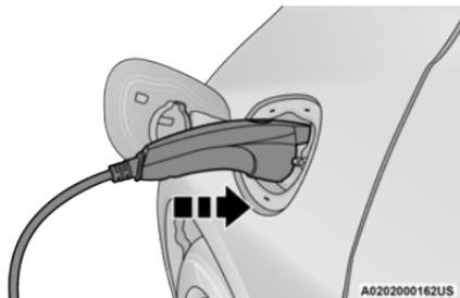
**Inserting The Charge Connector Into The Vehicle Charge Inlet**
