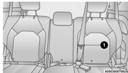
Routing The Rear Seat Belt Latch Plate
