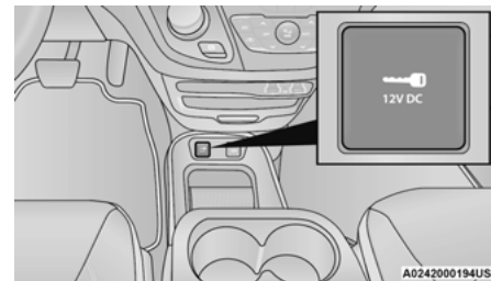
12 Volt Front Power Outlet (On Center Stack)
