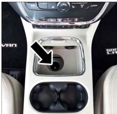
Winch Drive Nut Location
