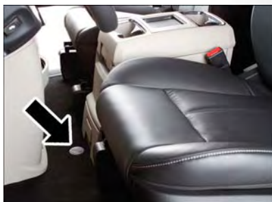
Winch Cover Location
