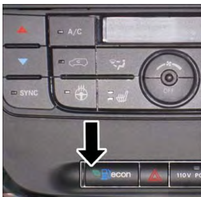
ECON Switch Location
