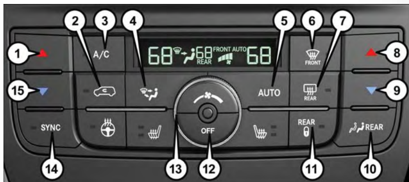
Three Zone Automatic Temperature Controls (ATC)
