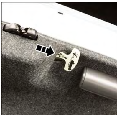
Trunk Emergency Internal Release
