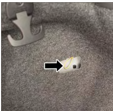
Fuel Door Emergency Release
