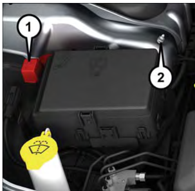
Remote Battery Posts
