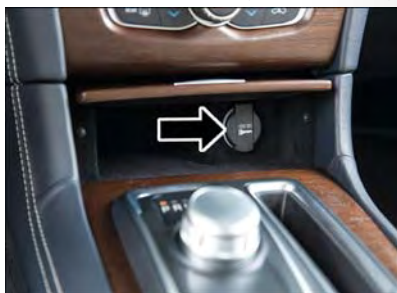
Front Power Outlet
