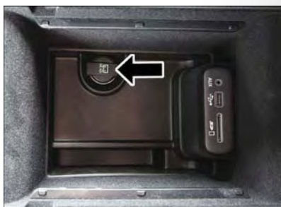
Center Console Power Outlet
