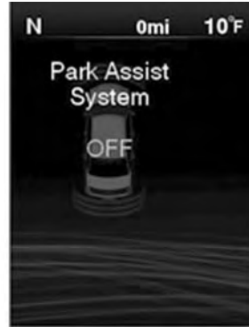
Park Assist System OFF
