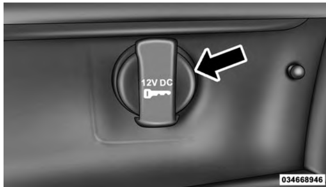
Front Power Outlet
