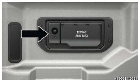
On-Board Power Panel
