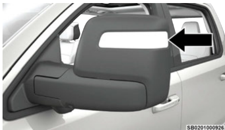
Forward Utility Light
