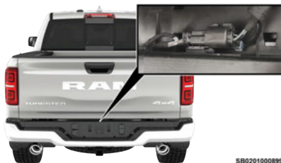
Wiring Harness Location
