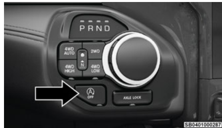
Stop/Start OFF Switch
