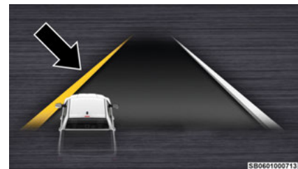
Lane Crossed (Flashing Yellow Line)
