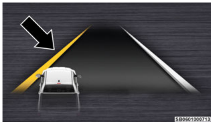
Lane Crossed (Flashing Yellow Line)
