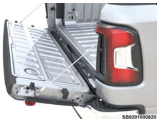
Tailgate Only Supported By Cables
