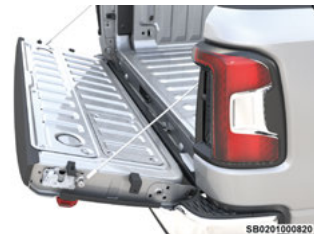
Tailgate Only Supported By Cables
