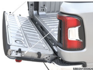
Tailgate Only Supported By Cables
