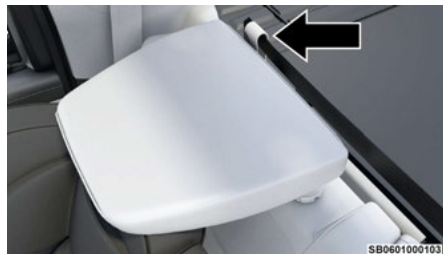
Outboard Tether Anchorage
