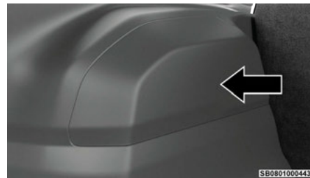
Rear Power Distribution Center Location
