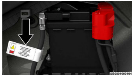
Negative Battery Cable Label Location
