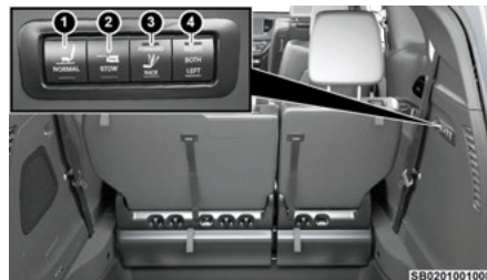
Rear Panel Power Switch Bank
