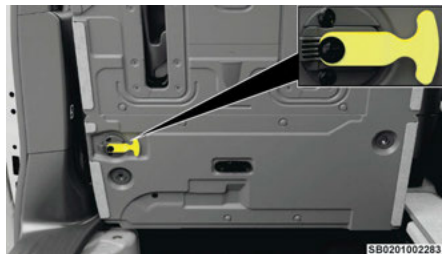
Storage Bin Cover Emergency Release Lever
