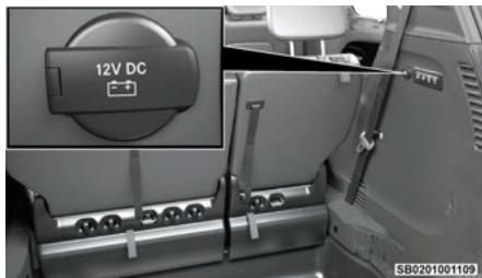
Rear Power Outlet
