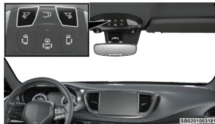
Courtesy Light Switches
