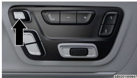
Power Four-Way Head Restraint Adjustment Switch
