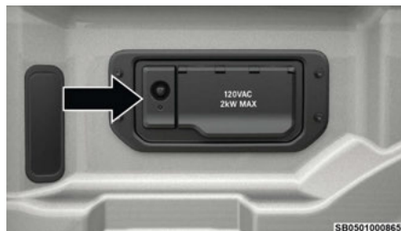
On-Board Power Panel
