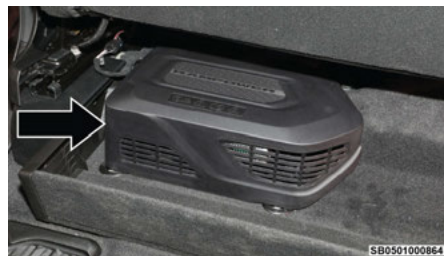
Power Panel Inverter Under Rear Seat
