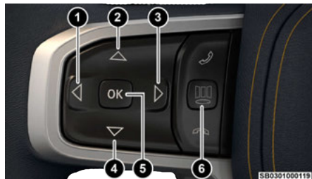
Instrument Cluster Display Control Buttons
