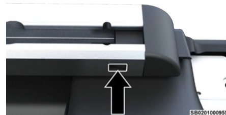
End Cap Release Button Without Tonneau Cover
