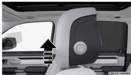
Upward Adjustment (Manual Head Restraint)
