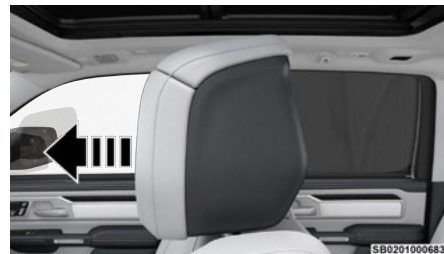
Forward Adjustment (Power Head Restraint)
