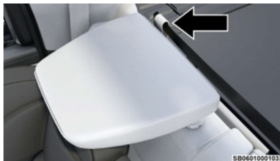
Tether Strap Through Outboard Tether Strap Loop
