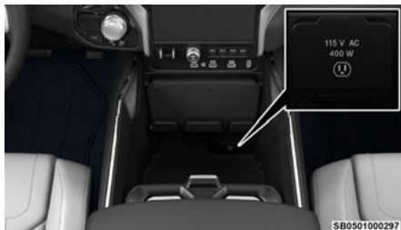
Center Console Power Inverter Outlet
