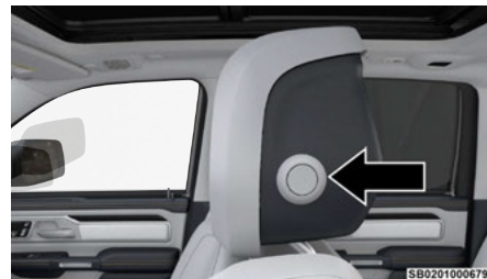
Manual Head Restraint Adjustment Button
