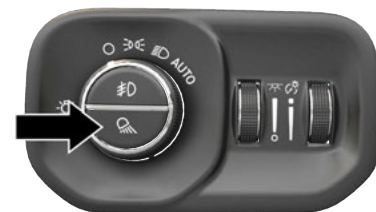
Cargo/Bed Lights Button On Headlight Switch
