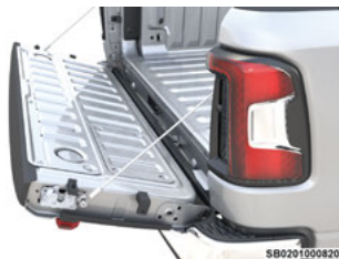
Tailgate Only Supported By Cables
