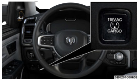
Instrument Panel Power Inverter Switch
