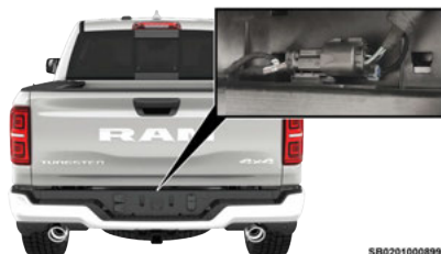
Wiring Harness Location
