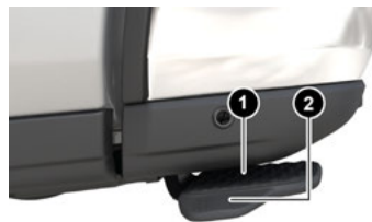
Bed Step Components (Standard Tailgate)
