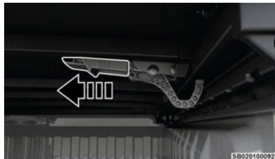
Slide Locking Lever Towards Inside Of Truck
