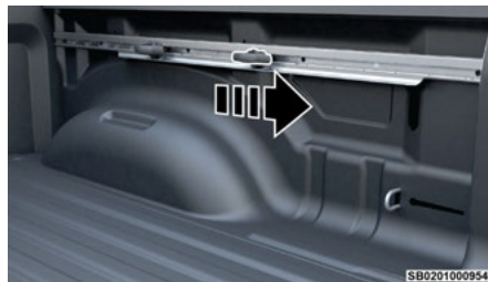
Slide Cleat Forward To Remove
