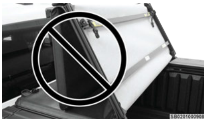
Incorrect Folding — Will Cause Damage
