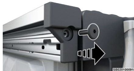
End Cap Screw Location With Tonneau Cover
