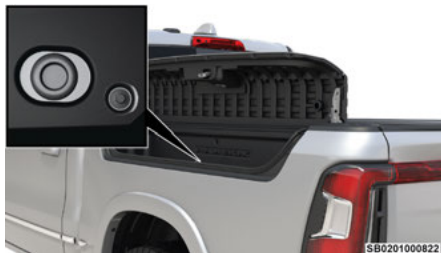
RamBox Drain Plug Removal
