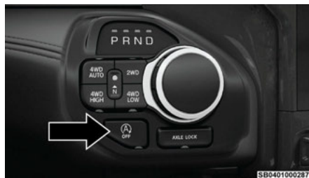
Stop/Start OFF Switch
