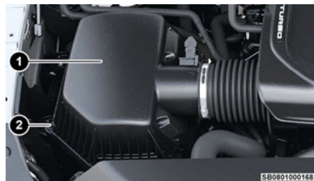
Engine Air Cleaner Filter — 3.0L SO Engine
