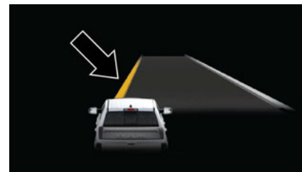
Lane Crossed (Flashing Yellow Line)
