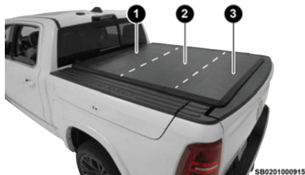
Position Two (Front And Rear Latches Latched)
