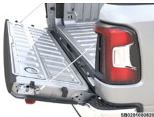
Tailgate Only Supported By Cables
