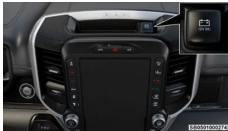
Power Outlet — Top Of Center Stack
