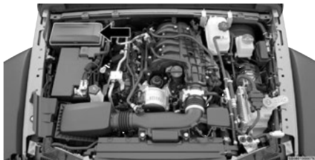
Power Distribution Center Location
