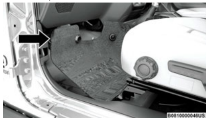
Front Carpet Pulled Away
