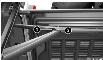
Wiper Blade Removed From Wiper Arm
