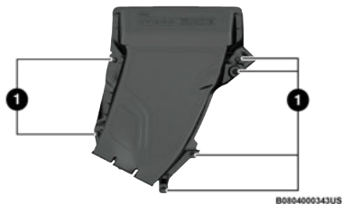
First Water Separation Chamber
