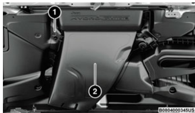
First Water Separation Chamber
