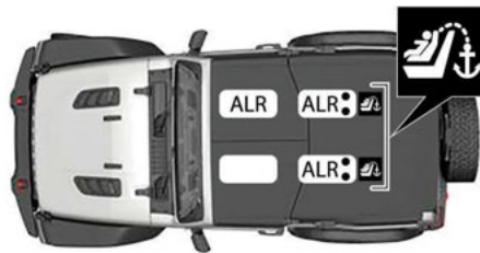
ALR — Switchable Automatic Locking Retractor Locations (Two-Door Models)
