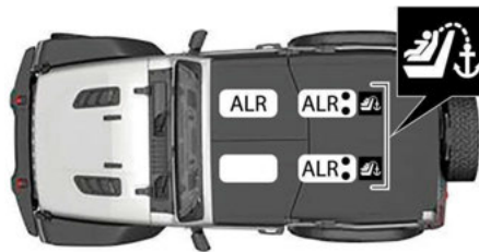
Automatic Locking Retractor Locations (Two-Door Models)
