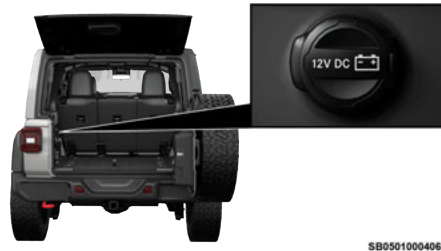
Rear Cargo Power Outlet
