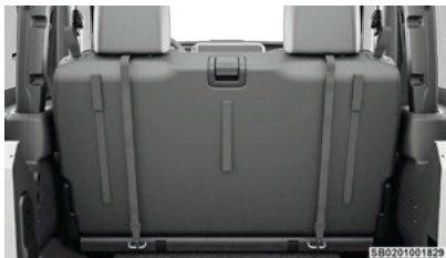
Tether Strap Mounting (Two-Door Models)
