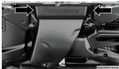
First Water Chamber Removal
