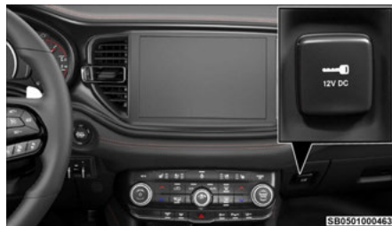
Front Power Outlet
