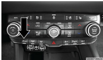
Stop/Start OFF Switch
