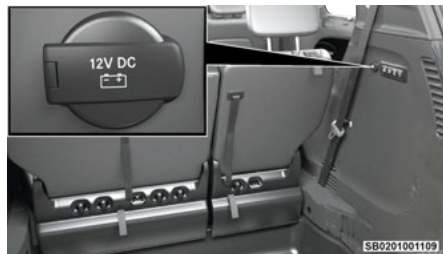
Rear Power Outlet
