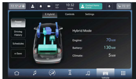
Power Flow Screen
