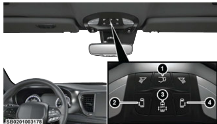
Overhead Console Power Switches
