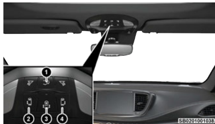
Overhead Console Power Switches
