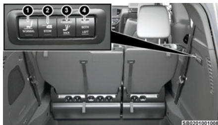
Rear Panel Power Switch Bank
