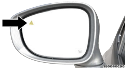
Warning Light Location
