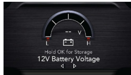
Storage Mode Activation Location
