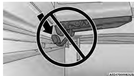
Improper Clamp Position
